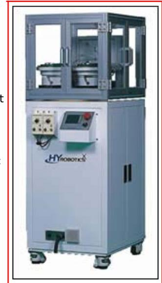
A new system from HYRobotics inexpensively orients and positions lightweight inserts on a fixture by blowing them through tubes. A robot then picks up the inserts and places them in the mold.
