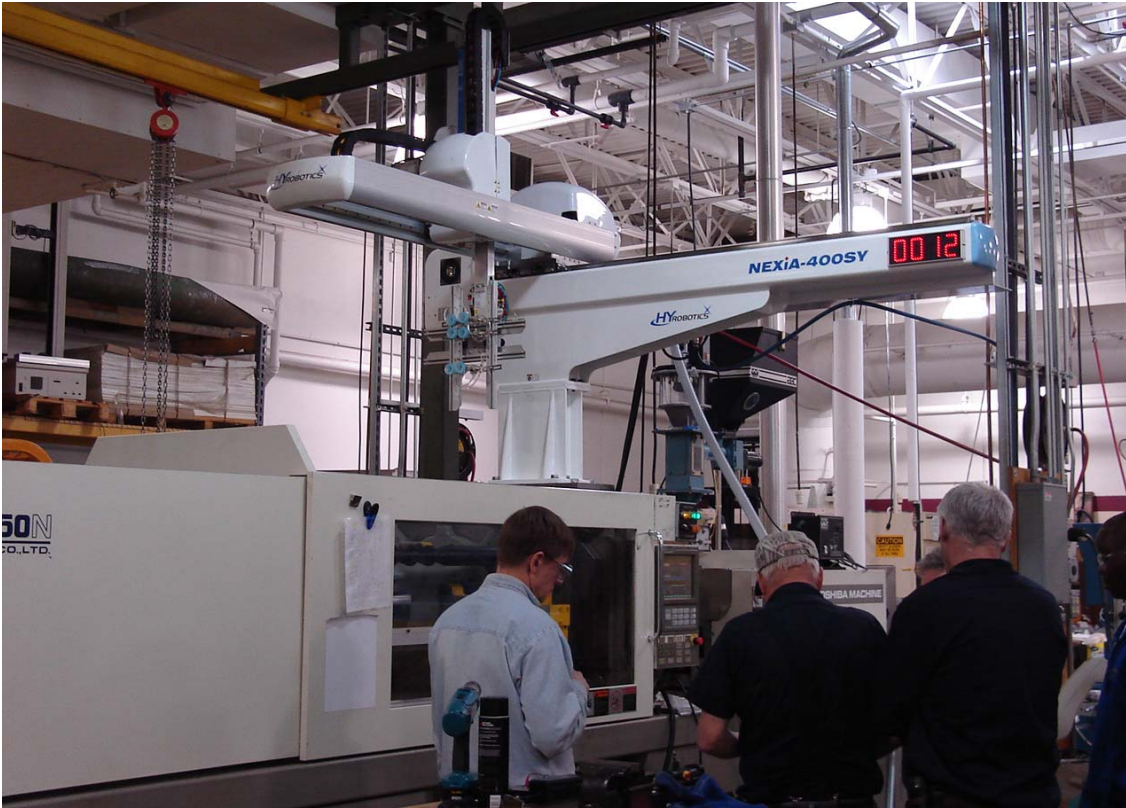
NEXIA-400S Installed on Toshiba 250 Tons IMM in Classroom.
