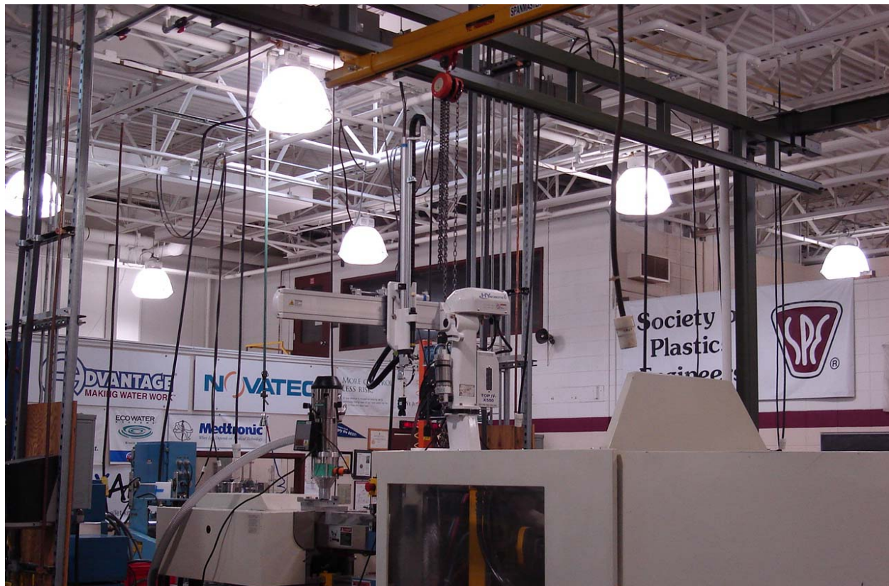
Simple Basic Pneumatic Style Sprue Picking Robot in Classroom : TOPIV Series.
