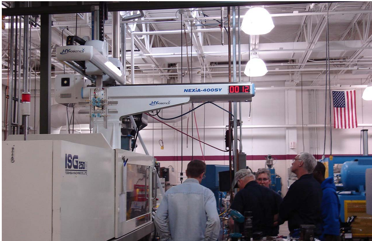
Picture shows Molding Machine and Robot are in Automatic Production for 12 Cycle in Classroom.
